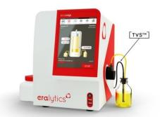
$\mathsf{TVS^{TM}} - \mathsf{D5191}$  Temperature Verification Sensor enables the specification of upper (and lower) temperature limits triggering an automatic warning if the sample temperature does not match the requirements. Thus the  $\mathsf{TVS^{TM}}$  is a very efficient tool helping you to save time and money for many reasons:
